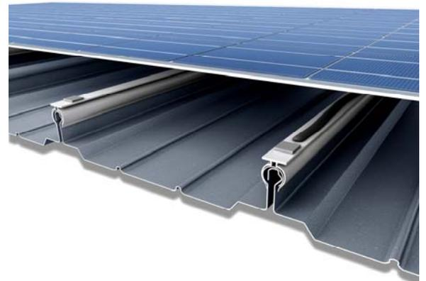
The SOLbond Seam system allows commercial and industrial buildings with standing seam roofs to be used for electricity generation. These roofs usually have a low load reserve, so the light SOLbond Seam system is the optimal solution. It is attached to rails that do not penetrate the roof membrane, and weighs only 11 kg/m<sup>2</sup>.
