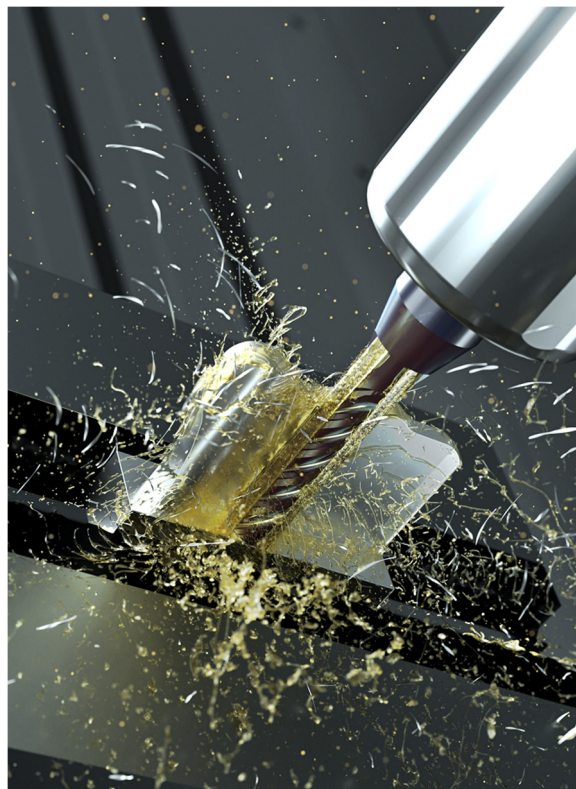
Cost-efficient machining from the solid of unalloyed titanium.
