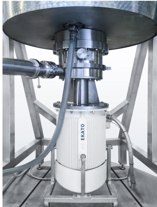
When looking especially at units with batch sizes of 5,000 liters or more, EKATO was lacking of an adequate homogenizer to handle the large amounts of product volume. While in laboratory or pilot plants the small volumes can be homogenized within minutes, the homogenization time on large machines always extended a lot due to the low throughput of the homogenizers related to the vessel volume.
