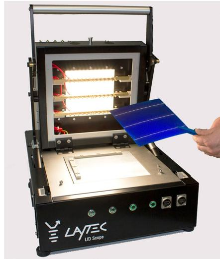
LID Scope degrades cells in a well-controlled procedure with electrical current and high temperatures by applying novel physical models developed by Fraunhofer Center for Silicon Photovoltaics (CSP) in Germany (patent pending). For the first time, cells can be degraded in a repeatable way, which means that LID Scope offers identical LID performance control from line to line and from lab to lab.
