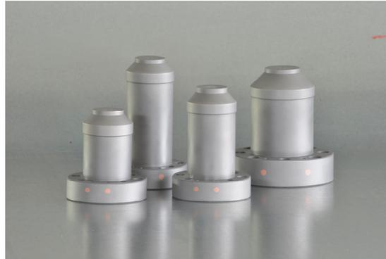
Unlike the previous production method, we now build the cooling part by laser sintering. This technique allows us to produce Gate Inserts parts with different diameters to meet your individual requirements. The moulding part can be fabricated with minimal oversize, keeping post-processing to a minimum. Leakage due to faulty solder joints is completely eliminated.
