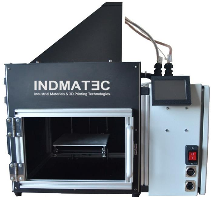
Following the successful printing of PEEK, the company introduced their first commercially available FFF 3D printer, 'INDMATEC HPP 155'. They are now expanding the printers' capabilities with a new 'Expert' level software package, which allows access to over 65 adjustable parameters, enabling users to print optimally with a range of high performance polymers, in addition to PEEK.
