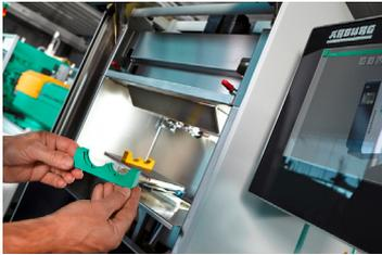
*Industrial additive manufacturing: with the Freeformer and Arburg Plastic Freeforming (APF), functional parts can be produced efficiently from qualified standard granulates without requiring a mould.*
