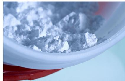
3M Glass Bubbles are used in many different areas. The tiny, high-strength hollow glass spheres are a popular fillers in paints, lacquers, adhesives and coatings, among other things. 3M has therefore carried out research in this area in the past years and has achieved significant advances in the Glass Bubbles technology.
