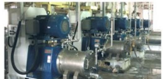
PNH SuperMaxZeta 60 agitator grinding mill (75KW)
