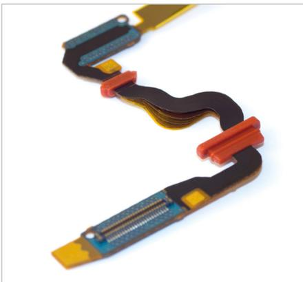
Multilayer flexible printed circuit with sealing and assembly
