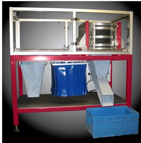
known products and innovations in the range of material. Collecting funnels, side safety curtains and butterfly curtains move parts gentle and safe and reduce rejects.
