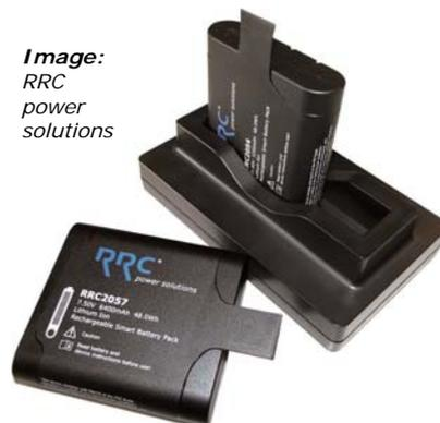
These are the latest Li-Ion battery packs from RRC power solutions which combine the highest energy density in the smallest package. One of the battery packs is the RRC2057, designed as a 2s2p configuration, provides 48 Wh of energy at 7.5 V and 6400 mAh. The RRC2054 has the same energy content (48Wh) and has a voltage of 15 V and a capacity of 3200 mAh in a 4s1p configuration. Both packs are compatible with SMBus and SBDS in accordance with the specification Rev 1.1.
